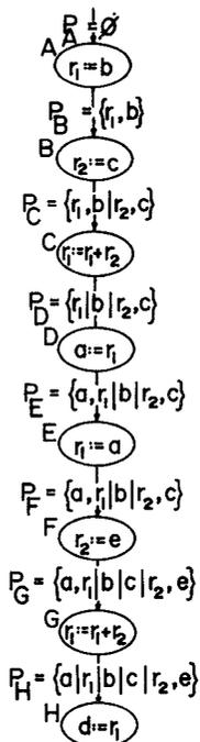
Figure 4. Elimination of redundant register load operations.
